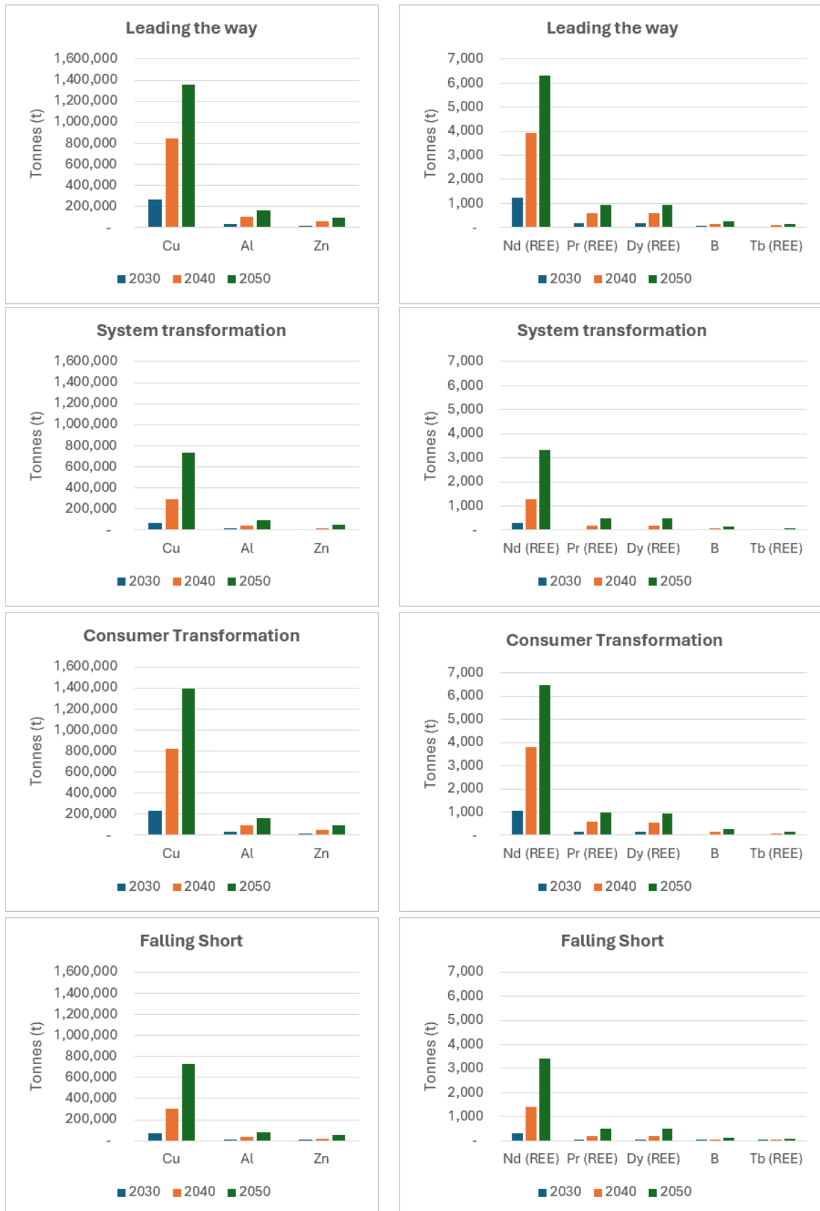
Figure 12: Cumulative forecast UK heat pump demand (tonnes) for the materials considered in this study between 2020 and 2050 under four different scenarios: Leading the way (LW); System transformation (ST); Consumer transformation (CT); and Falling short (FS).
