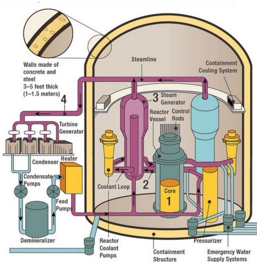
**Figure 2** Salient components of a PWR (Nuclear Regulatory Commission, 2023). © NRC
