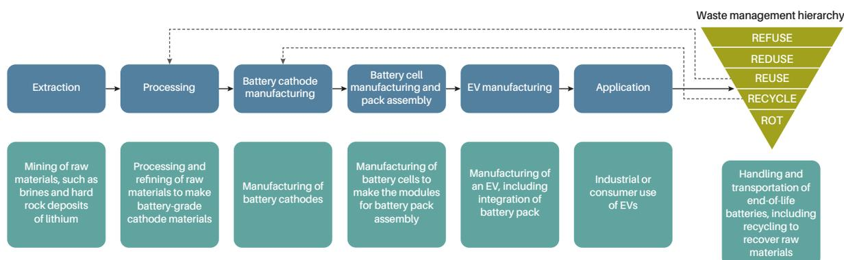
Figure 8 A generic battery mineral supply chain. BGS © UKRI.
