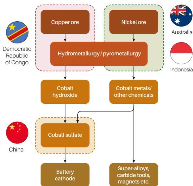
**Figure 11** Cobalt value chain. The flags denote the principal countries in which selected parts of the value chain are concentrated. Reproduced with permissions. Source: IEA (2022a) *The Role of Critical Minerals in Clean Energy Transitions*, World Energy Outlook Special Report. All rights reserved.
