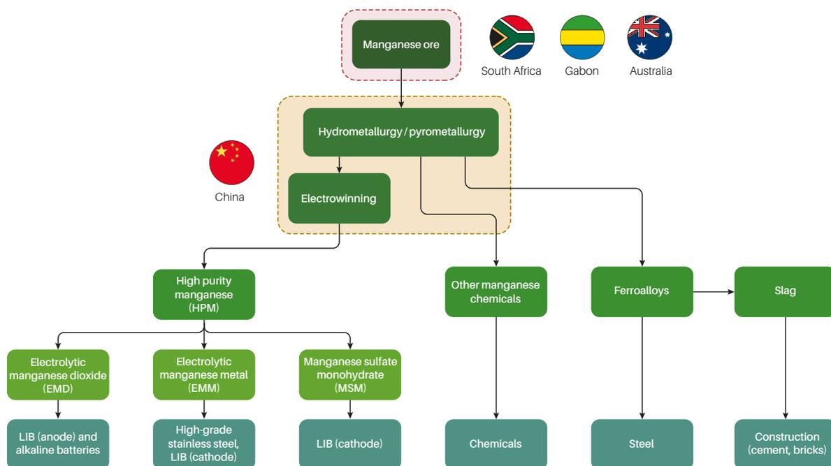
**Figure 12** Manganese value chain. The flags denote the principal countries in which selected parts of the value chain are concentrated. BGS © UKRI.
