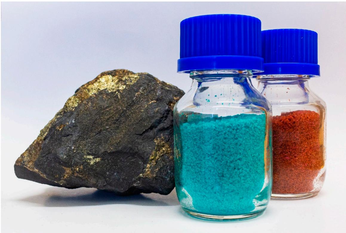
Figure 14 Nickel-copper-cobalt ore and its end-products nickel (blue) and cobalt sulfates (orange) produced at the Sotkamo mine in Finland operated by Terrafame. The mine produces these chemicals used for battery technologies on-site. The Sotkamo mine has the largest cobalt resources and reserves in Europe, that are currently in production (© Terrafame Ltd. 2020<sup>84</sup>).
